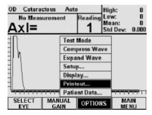
**Figure V-O** Selecting Printout from the A-Scan options menu.
