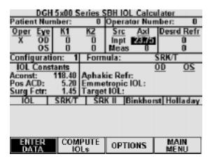
**Figure V-T** Accessing the IOL calculator and inputting a valid axial length.
