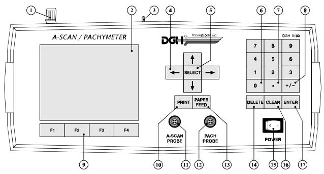
Figure III-A DGH 5100 front panel layout.
