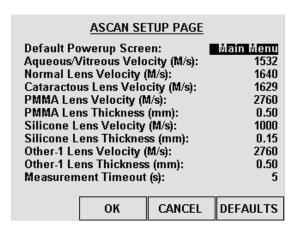
**Figure V-B** A-Scan Setup page.
