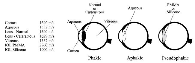
Figure I-E Speeds of sound for ophthalmic structures.
