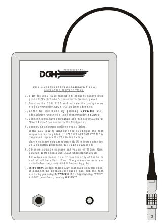
**Figure III-D** Electronic Calbox used for checking Pachymeter calibration.
