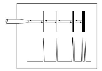
**Figure I-A** Sound hitting an interface perpendicularly.
