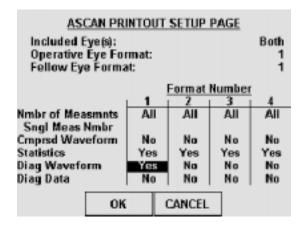
**Figure V-P** Enabling the Diagnostic Waveform for printout format #1.
