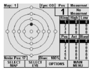
**Figure VI-L** Pachymeter ready to take a measurement at Position 1.
