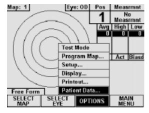
**Figure VI-C** Accessing the Patient Data Input page from the Pachymeter mode.
