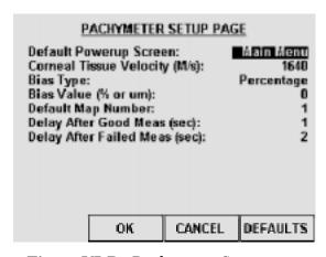
Figure VI-B Pachymeter Setup page.
