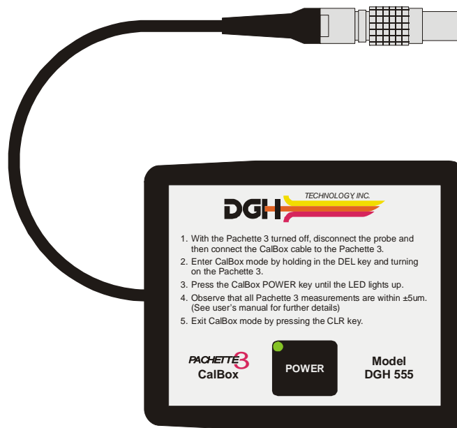
Figure III-E DGH 555 Pachette 3 Electronic CalBox
